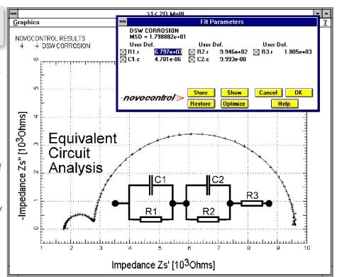
Equivalent circuit analysis supports definition of arbitrary RLC networs in combination with any user-defined complex function such as, e.g.,  $sin(w\cdot(var1+j\cdot var2))$ .
